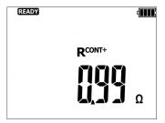
R<sub>CONT+</sub> – resistance measured with 200 mA positive polarity current
