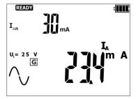
Read the main measurement result:  $I_A$  current.
