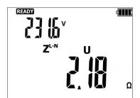
Read the main result: the fault loop impedance  $Z_{\text{\scriptsize S}}$  and the mains voltage during the measurement.
