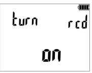
Reset the tested RCD after each tripping.
