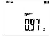
R<sub>CONT</sub>- – resistance measured with 200 mA negative polarity current
